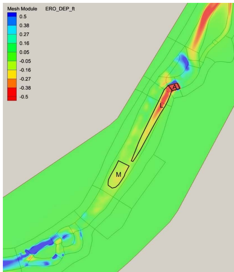
Figure 51. Modeled aggradation and degradation for injection of 2,000 yd 3 of coarse sediment. Aggradation is positive and degradation is negative. The sediment drop zone area is labeled “A,” the location of the new lateral bar is labeled “L,” and the incipient medial bar is labeled “M.”
